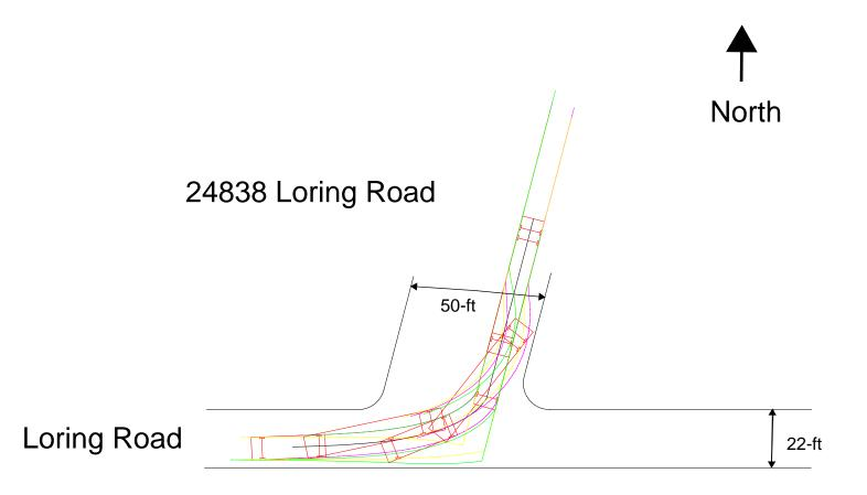
Tri-Hull Crane Turning Template
